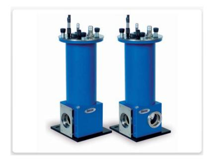
The Variable Temperature Cell Holder is the ideal accessory to use for the transmission study of liquid or solid samples at temperature range from -190°Cand 250°C. The temperature achievable will be dependant on the type of sample cell used.
